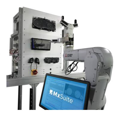
**Other Vehicle Functions** – The test system uses a precision power supply to test the response of the infotainment system under quickly changing power conditions, such as vehicle startup, accessory operation, and driving conditions. A diagnostic tool automatically scans the ECUs, saves the scanned file, and imports the information into the test report.
